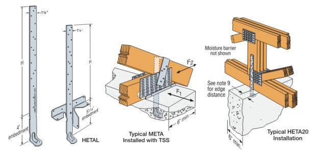
FIGURE 3: META / HETA / HHETA / HETAL Dimensions and Installation Details
