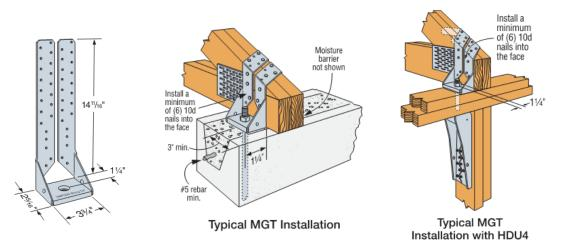
FIGURE 9: MGT Dimensions and Installation Details
