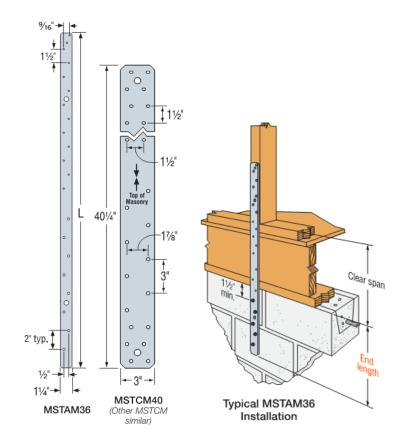
FIGURE 5: MSTAM / MSTCM Dimensions and Installation Details
