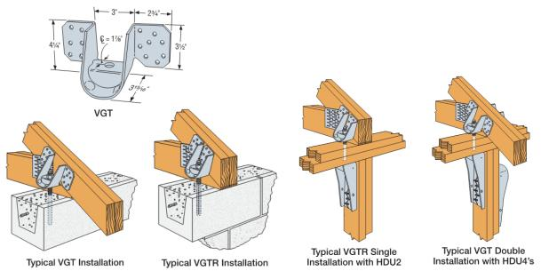
FIGURE 10: VGT / VGTR / VGTL Dimensions and Installation Details
